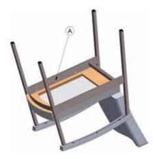
**A:** Turn the chair upside down and remove the upholstered seat cushion by removing the four #2 Philips screws.
