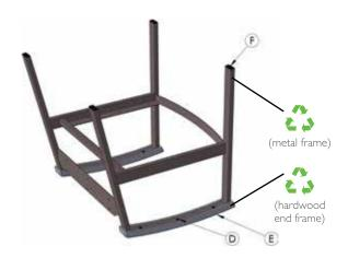
**D & E:** Place the chair upside down or on its side. Next, using the #2 Phillips screwdriver, remove the three screws attaching each arm cap to the frame. Take the flat blade screwdriver and hammer knock out the glide free from each leg.
